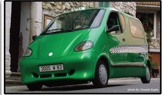
2010 Going Green Tata Motors of India is developing the Air Car. It runs on compressed air and is emission free.
